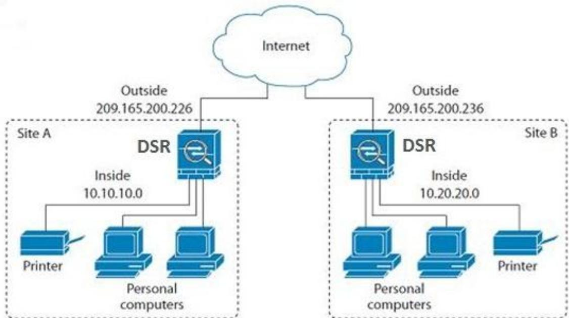
**Figure 54: Example of three IPsec client connections to the internal network through the DSR IPsec gateway**
