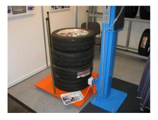
⇒ Additional inclined access-ramp on the 3 open sides of the loadplatform.
