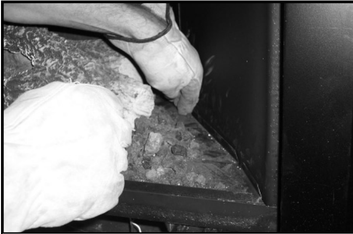
Figure 7 Move Lava Rock to Install Side Refractory
