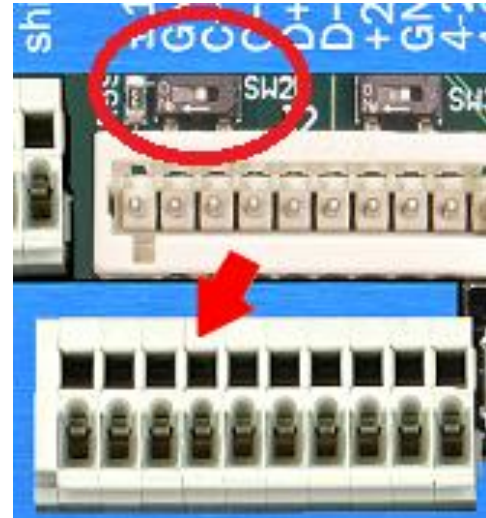
Figure 8 SSI Termination Resistor Switch
