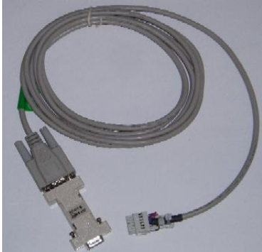
Figure 16 Photograph of MR232-1 RS422/RS485-to-RS232 Adapter Cable.
