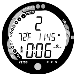
Fig. 60 - Immediate Violation Gauge Mode (after surfacing)
