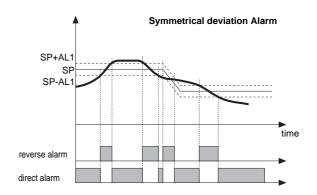
For AL1 = Symmetrical Lo deviation alarm with Hvst 1. AL1 t = 7 For AL1 = Symmetrical Hi deviation alarm with Hyst 1, AL1 t = 6
