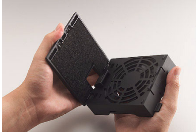
Figure 3.6: Replacing the fan filter
