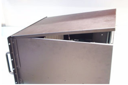
Figure 2.5: Removing the top chassis cover
