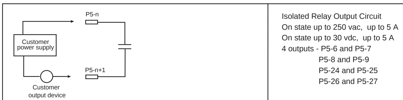
Figure 4.24 Typical Isolated Relay Output Connections
