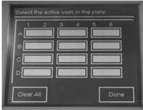
4. The user may select to **Clear All**, or clear each two sample position by touching the appropriate sample block. The sample pair will go dark, indicating that it is no longer selected.
