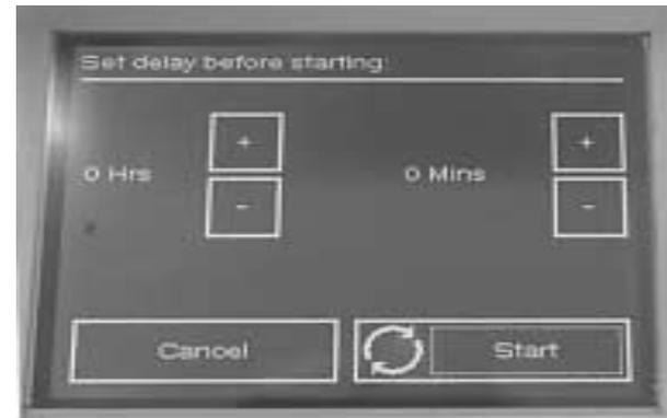
2. The start of the run can be delayed up to 23 hours and 50 minutes. This will enable the user to time the digestion to end whenever desired.
