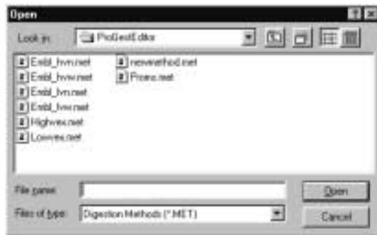
2. Select (highlight) the desired protocol and select **Open** to bring the protocol into the *ProGest Digestion Method Editor* window.
