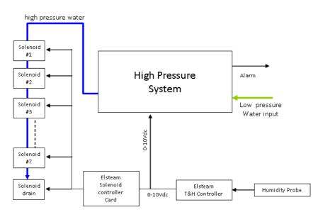
the humidistat (0-10V) controls the solenoids controlled card (for proportional working mode) as well as the activation (threshold set at 1V) of the high pressure system.
