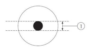
If oil level is not within  $\mathbb O$  zone, add or remove oil in the tank. Check for oil leaks.
