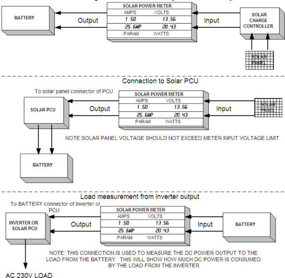
Solar Charge Controller Connection [NOT SOLAR PCU]
