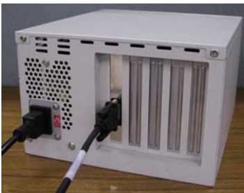
Figure 2.9. Plugging the power cable into the ECH-PE-CE-F4A
