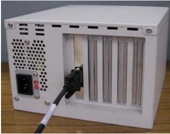
Figure 2.8. Connecting the connection cable to this product
