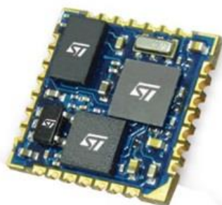
Figure 16 – iNemo M1 System-on-Board with the STM32 uC
