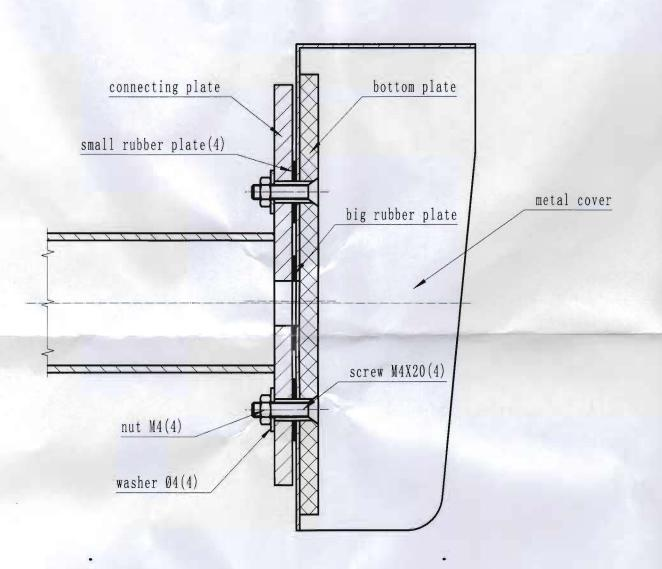
LM106 Wired Keypad Assembly Diagram
