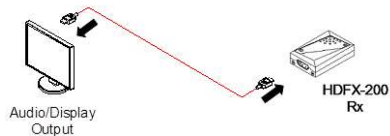
Figure 5 – Connection of HDMI copper cable between Receiver and display
