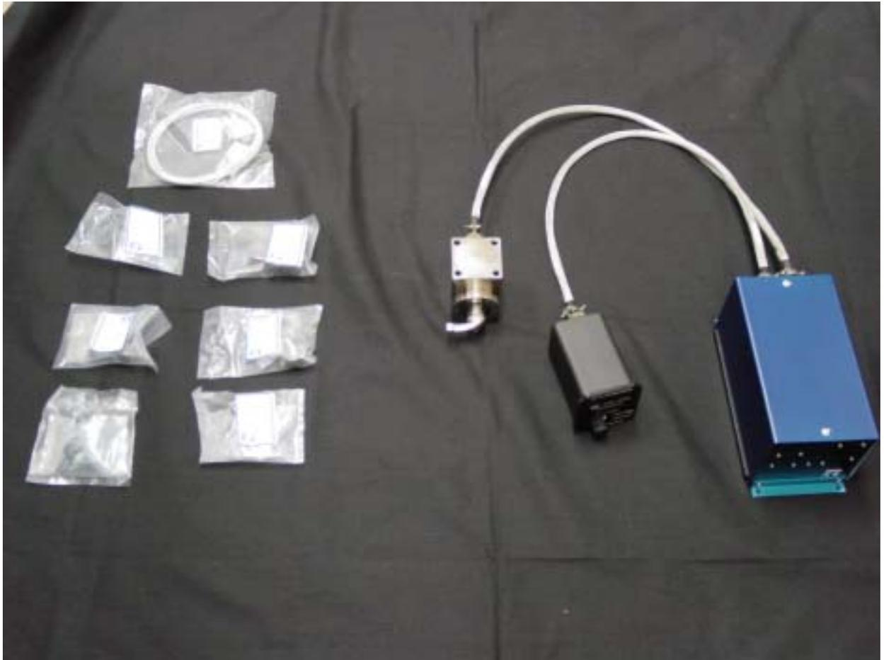
Figure 17. 1011C Hygrometer Complete
