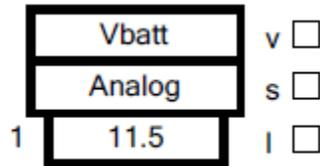
This feature is not functional on powerONE before version 5. In earlier versions, Vbatt can be monitored by connecting it to a UserIO configured as an analog input.
