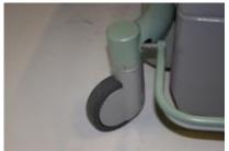
The chair has four large wheels: the two front wheels are fixed, and the two rear wheels are steerable. This makes the chair easy to move and steer.
