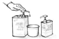
Figure 2 Dispense the proper proportion of resin and hardener.
