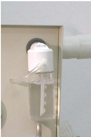
Fig. D Symptom of clogged nebulizer
