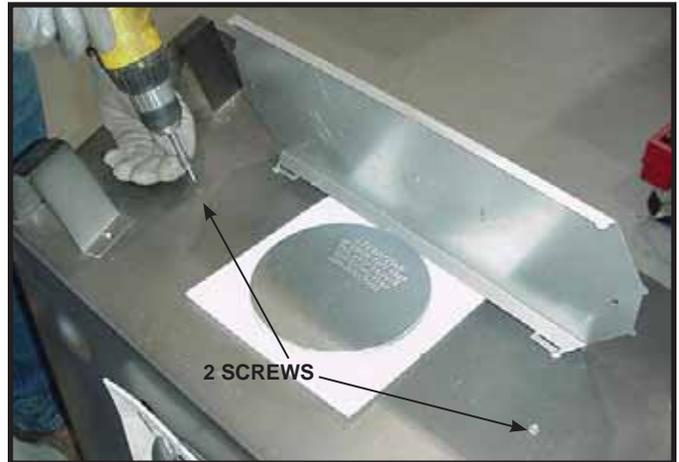
**Figure 7.3** Replace the two screws as shown.
