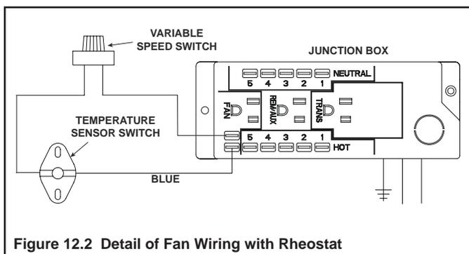
Figure 12.2 Detail of Fan Wiring with Rheostat
