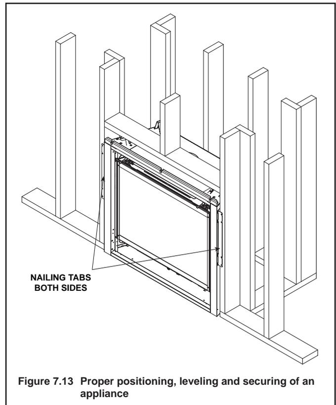
Figure 7.13 Proper positioning, leveling and securing of an appliance
