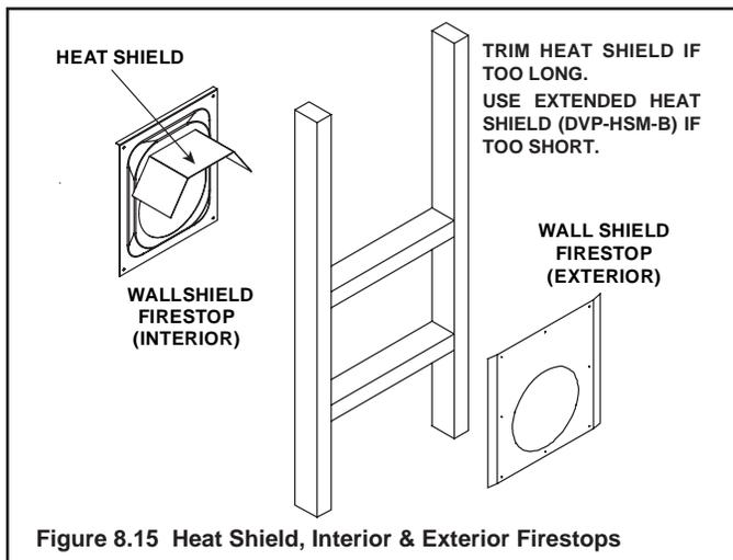
Figure 8.15 Heat Shield, Interior & Exterior Firestops
