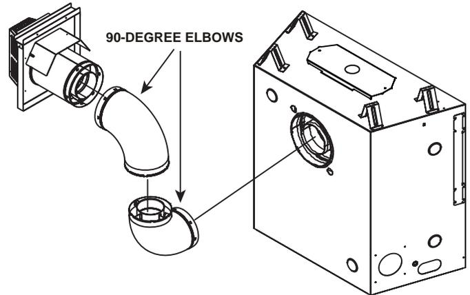
Use two 90° elbows for corner installations. The use of two 90° elbows in a corner installation will affect space requirements.
