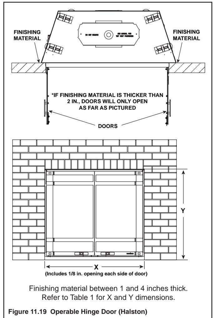
Figure 11.19 Operable Hinge Door (Halston)
