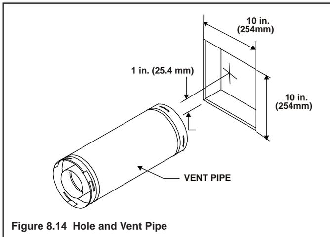
Figure 8.14 Hole and Vent Pipe
