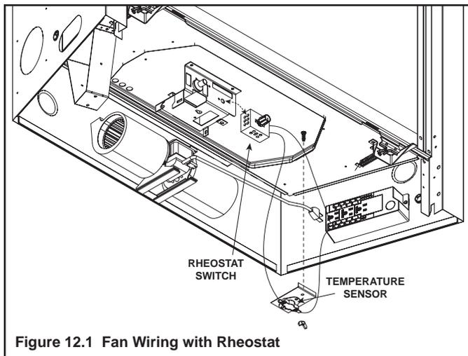
Figure 12.1 Fan Wiring with Rheostat
