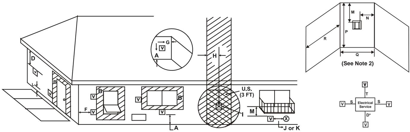
**V** = VENT TERMINAL      **X** = AIR SUPPLY INLET      = AREA WHERE TERMINAL IS NOT PERMITTED
