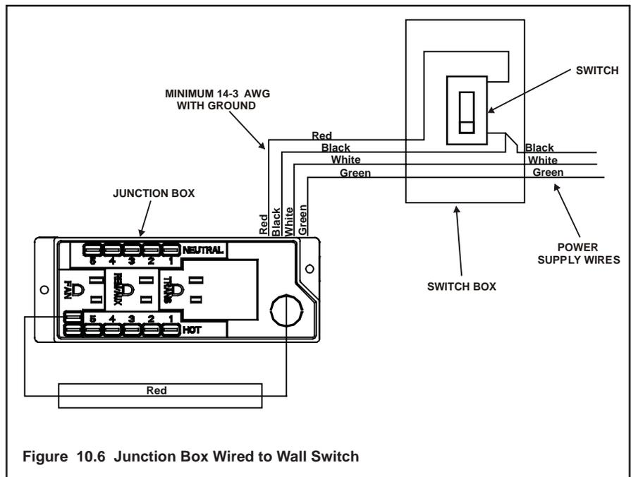
Figure 10.6 Junction Box Wired to Wall Switch
