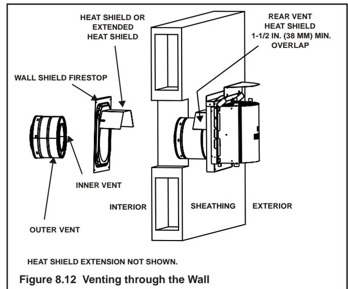
**Note:** Where required, an exterior wall flashing is available. When penetrating a brick wall, a brick extension kit is available for framing the brick.
