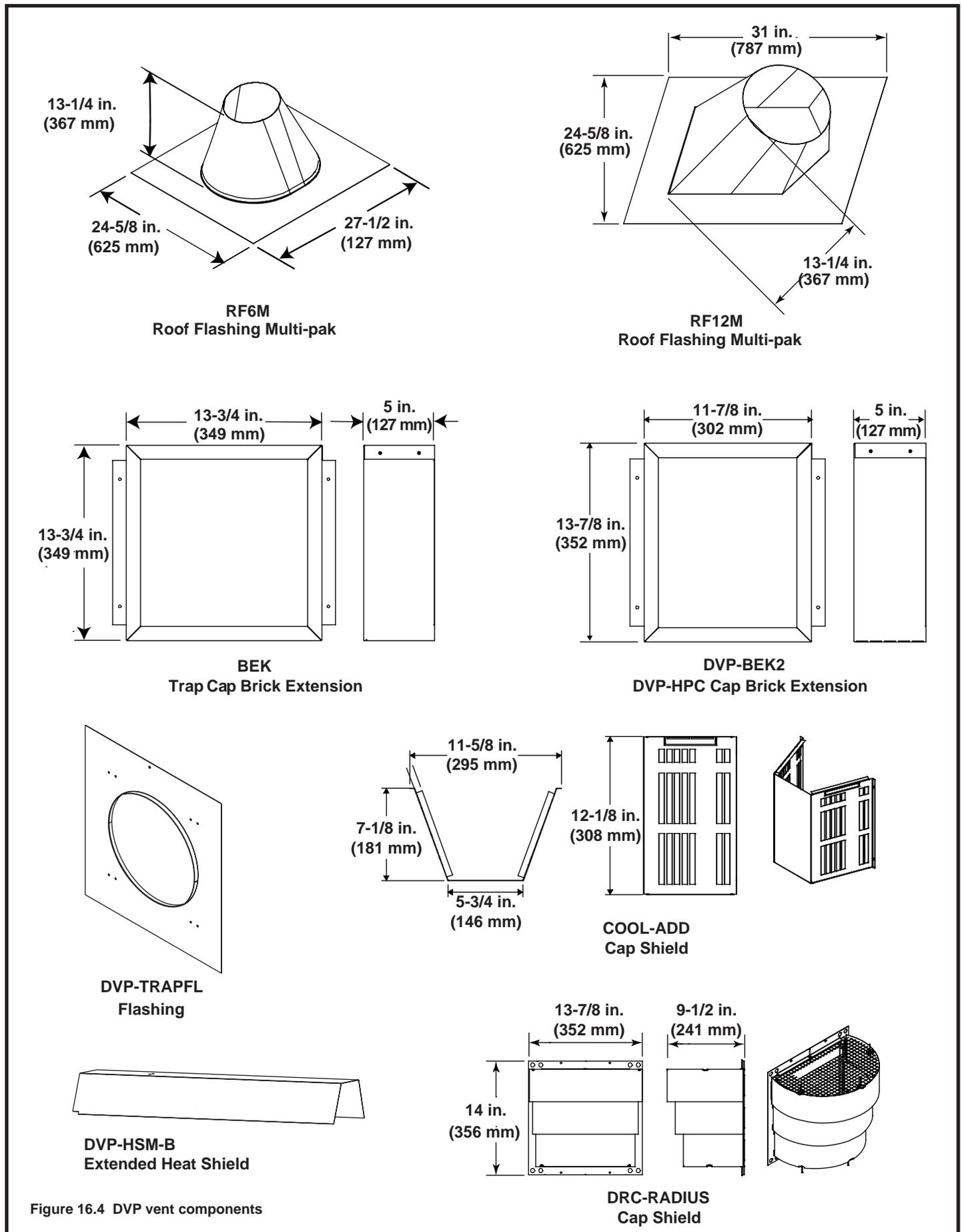
Figure 16.4 DVP vent components
