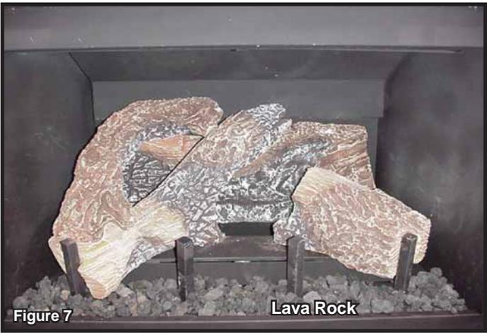
**Log #4 (SRV2113-703):** Locate the notch on the bottom of log # 4. Mate the notch with the shoulder screw that is located on the burner top. Mate the rear groove with the far right grate tine as shown above. Apply the supplied lava rock as shown above.
