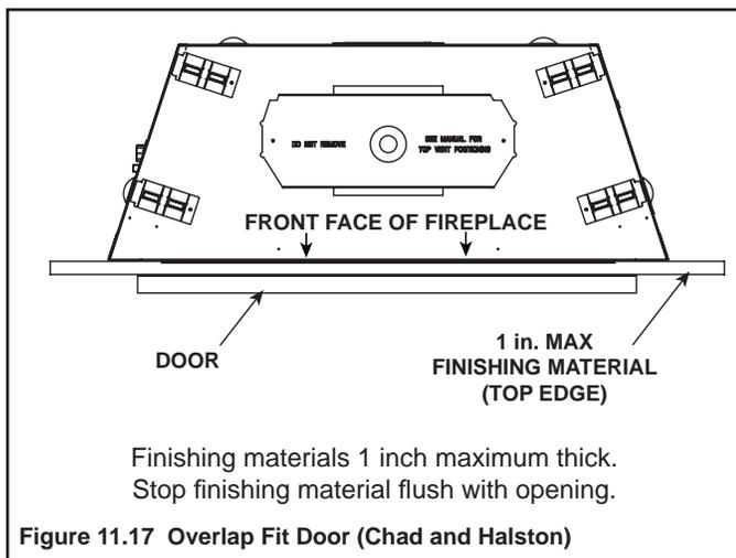
Figure 11.17 Overlap Fit Door (Chad and Halston)
