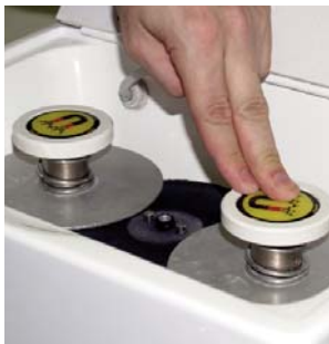
Press down handles to insure complete magnetic lock.
