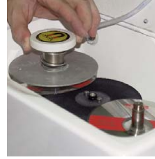
Place an Easy Load Handle on the discs
