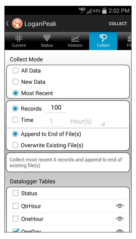
Collected data files are stored on your device in the Campbellsci/Data/name directory, where name is the name given to your datalogger when it was added to the LoggerLink App. With your device connected to a computer as a disk drive, you can navigate to this directory to copy your data files to the computer.
