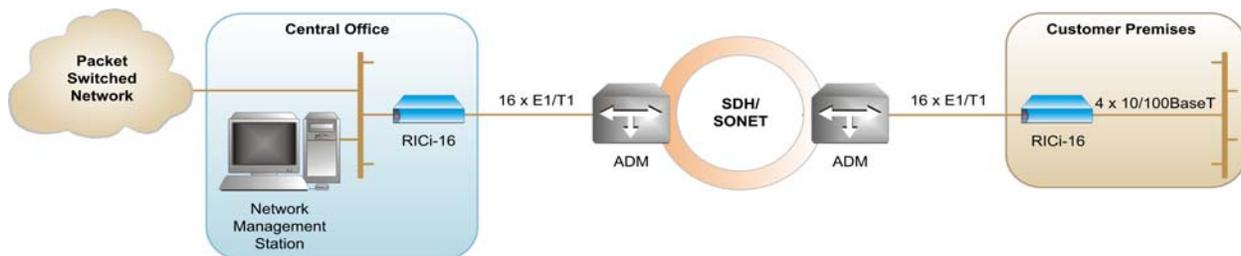
*Figure 1-1. RICi-16 Extends Ethernet Services over Multiple E1/T1 Circuits*
