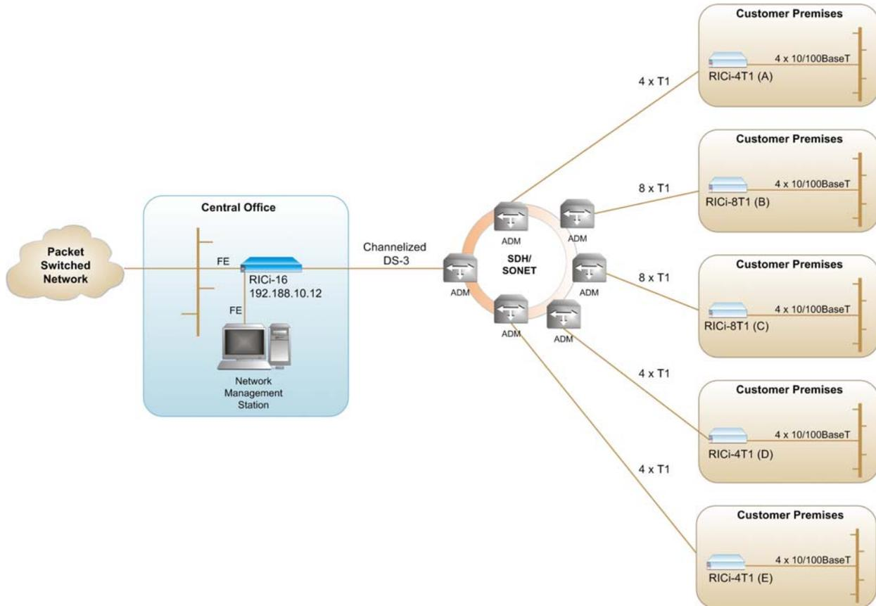
*Figure 5-20. RICi-16 with Channelized DS-3 Supporting Multiple Customer Premises*
