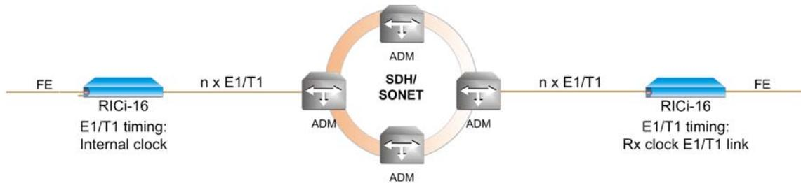
Figure 1-9. E1/T1 Clock Configuration for RICi-16 Working Opposite RICi-16
