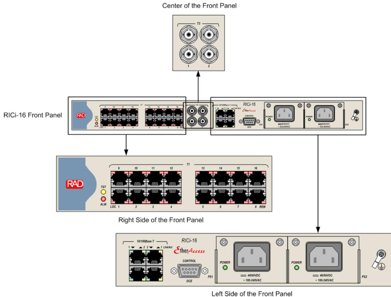
Figure 3-1. RICi-16 Front Panel with T3 Connectors – Magnified
