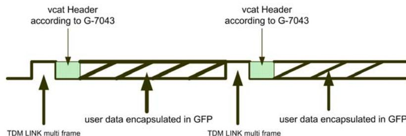
Figure 1-5. GFP Mapping over the PDH Signal
