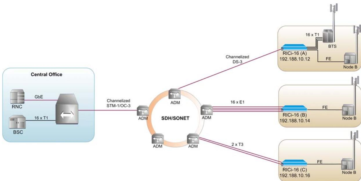
*Figure 5-1. Ethernet Cellular Backhauling over PDH/SONET/SDH*
