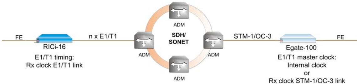
Figure 1-10. E1/T1 Clock Configuration for RICi-16 Working Opposite Egate-100
