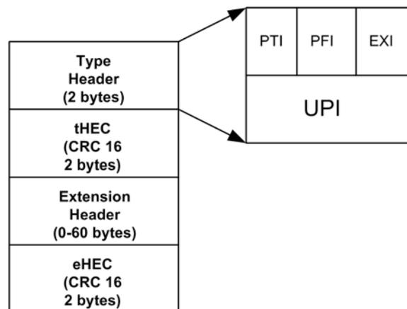
Figure 1-4. GFP Encapsulation - Payload Area
