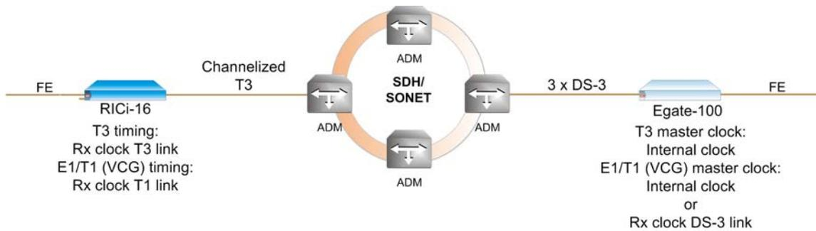
Figure 1-12. T3 Clock Configuration for RICI-16 Working Opposite Egate-100
