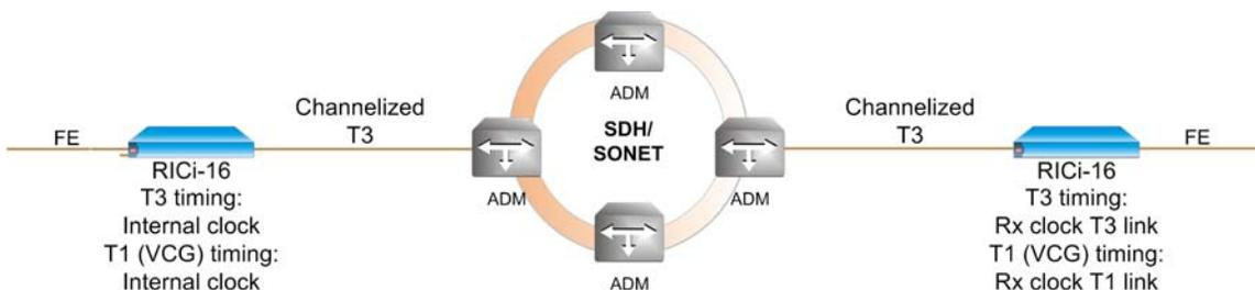
Figure 1-11. T3 Clock Configuration for RICi-16 Working Opposite RICi-16
