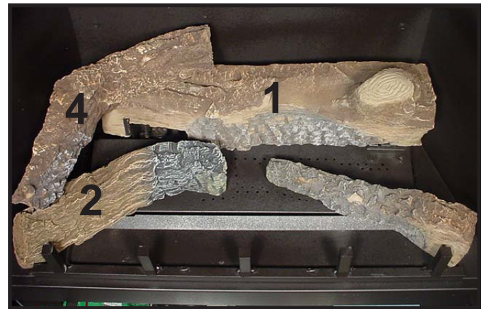
LOG #4 (SRV530-716): Place the left end of log #4 in the groove on log #2 and the right end on log #1 as shown.
