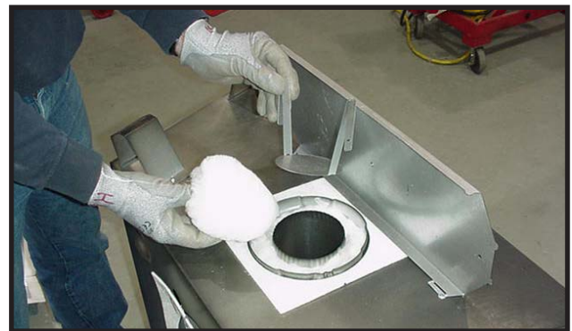
Figure 20. Remove the insulation basket and white insulation from the center flue pipe.
