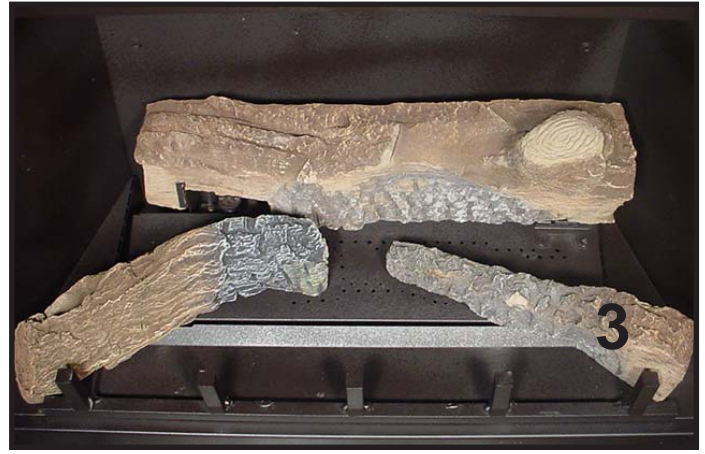
LOG #3 (SRV705-703): Rest log #3 against the right front grate corner and place its slot over the right burner tab.
