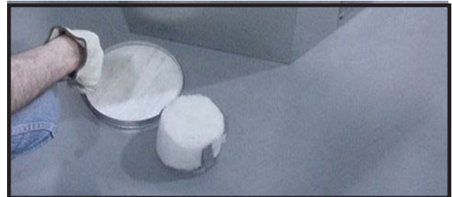
Figure 26. Discard the flue cap, remove and discard the insulation basket. Note: Once the flue cap has been removed it CANNOT be reattached.
