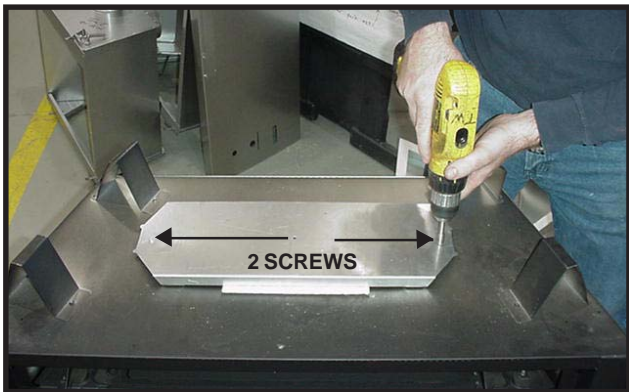
Figure 16. For top flue, remove the two screws holding the top heat shield in place. For rear flue, see next page.
