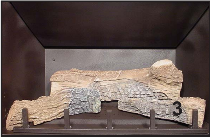
LOG #3 (SRV705-703): Rest log #3 against the right front grate corner and place its slot over the right burner tab.
