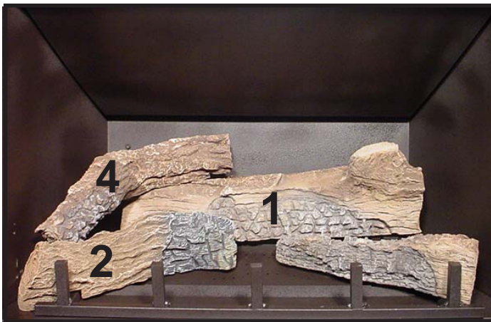
LOG #4 (SRV530-716): Place the left end of log #4 in the groove on log #2 and the right end on log #1 as shown.
