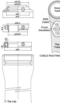
2. Compression Ring 3. 1" Cartridge Bearing 4. Crown Race
