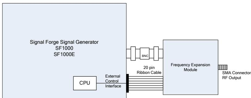
Figure 4. Connecting the 1800M to the Signal Forge 10x0 Signal Generator
