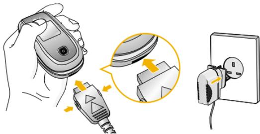
1. With the arrow facing you as shown in the diagram push the plug on the battery adapter into the socket on the bottom of the phone until it clicks into place.
