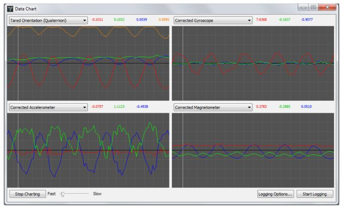
This tool provides various visualizations of the data that can be read from the 3 Space Sensor as well as the ability to log this data to a file.
