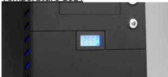
Temp. LCD which can be use for chassis's internal temp. monitoring.
