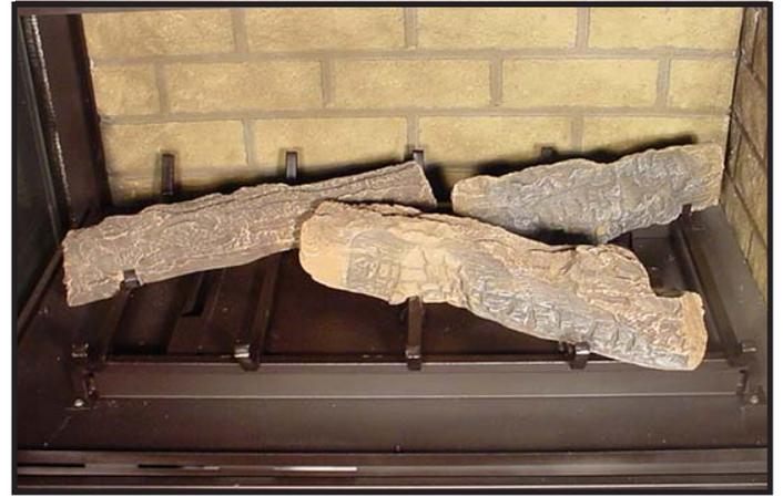
**LOG #3 (SRV2068-702):** Position log #3 across the first, second and third grate bars and pull towards the front against the grate tabs on bars one and three.
