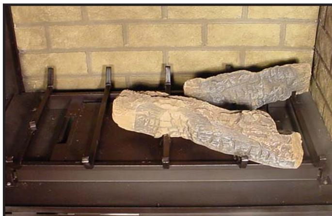
**LOG #2 (SRV2068-701):** Locate log #2 in right rear corner of the log grate using bottom grooves for placement. Place log against grate tabs on fourth and fifth bars.
