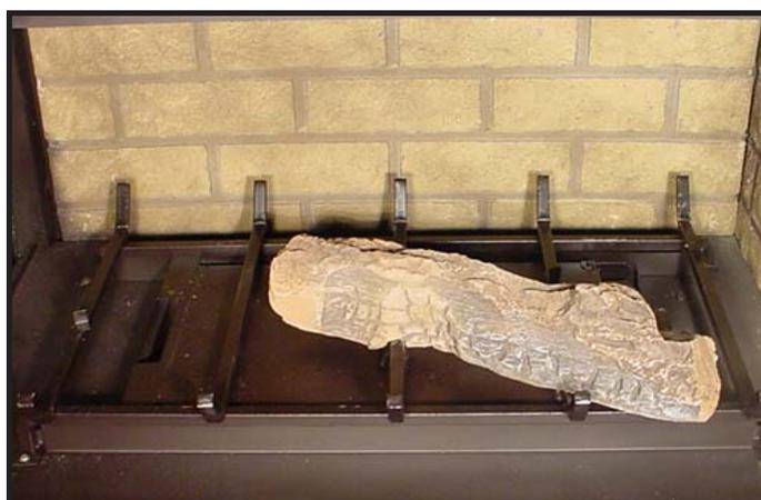
**LOG #1 (SRV2068-700):** Place log #1 in front of grate tabs on the third and fourth grate bars on the right front corner. Position so that the bottom grooves fit over bars and the log is snug against the grate tabs.
