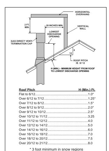
Figure 4.1 Minimum height from roof to lowest discharge
