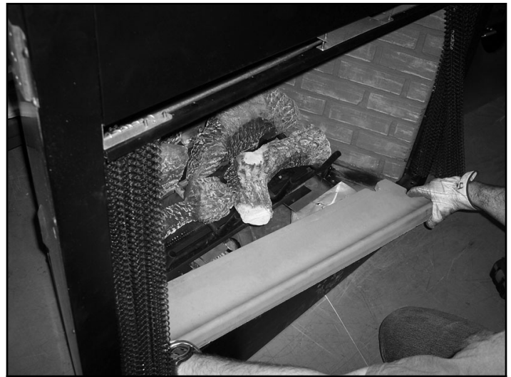
Figure 12.11 Remove Hearth Refractory - Step 2
