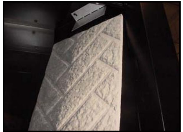
Figure 8 Sliding the Side Refractory Behind the Bracket (right side shown)
