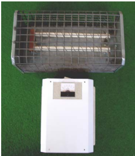
Dump Load and Controller
