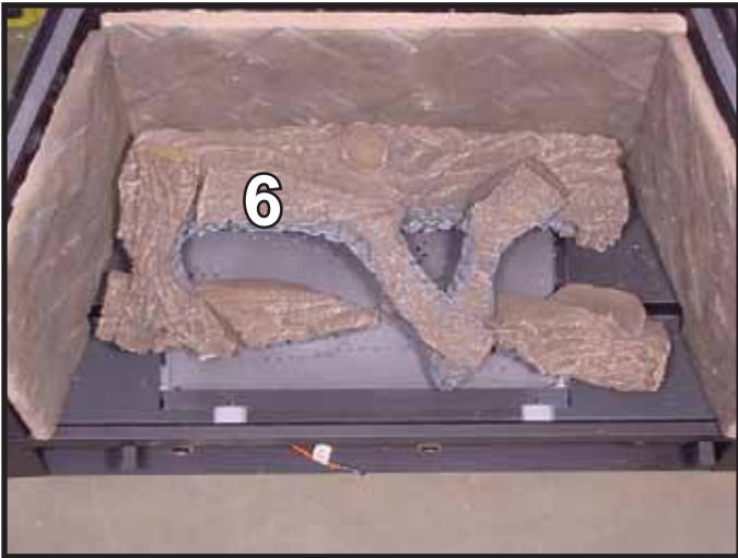
Log #6 (srv340-705): Place log #6 across log #1 and log #5. The notch in the bottom of log #6 rests in the carved out section on top of log #5 and the left end of the log sits in the horizontal carved out section of log #1.
