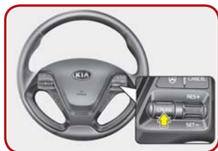
Cruise control system* [5] ON-OFF button to turn the system on
