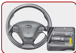
Set cruise control speed by pushing the SET-switch
