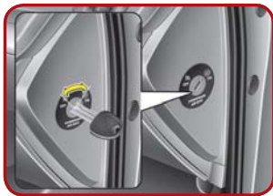
Passenger's front air bag ON/OFF switch* [3]
