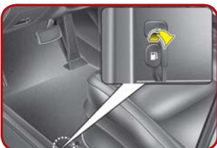
Opening the fuel filler lid Pull up fuel filler lid opener located on the driver's seat.
