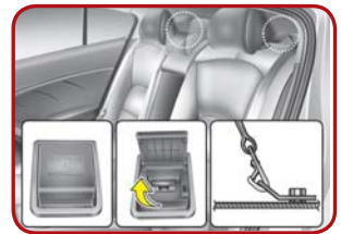
Securing with "Tether Anchor" system* [3]
