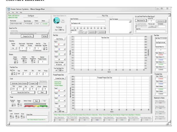
The Wave Gauge interface software is available from Ocean Sensor Systems and contains all of the features necessary to, configure, monitor and display raw and processed wave data or even upload small test files. It will run on most Windows based machines. The free Interface Program is available to downloaded and install on a PC from the Ocean Sensor Systems web site.
