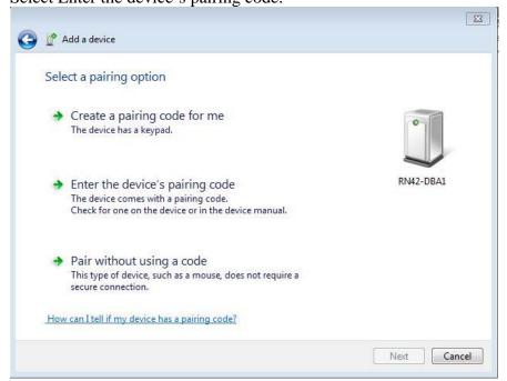
Enter the Wave Gauge Blue pairing code. 1234 is the pairing code for the unit when it
