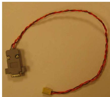
**Caution:** To convert the various voltage levels, a MAX232 is already set up in the POB-EYE module. The values Tx, Rx and GND are showed from a computer point of view.
