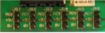
The connectors are plugged to pin RC0, RC1, RC2, RC3, RC6, and RC7 of PORTC.
