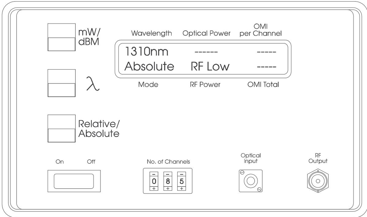
**Figure 2 The FOS 1000A after Initial Power-Up**
