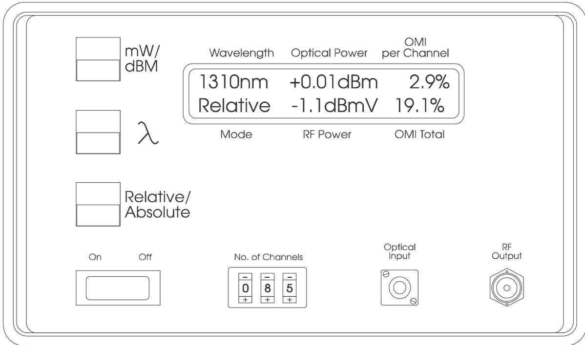
**Figure 10 The FOS 1000A Relative Display Mode, with RF Modulation Change**
