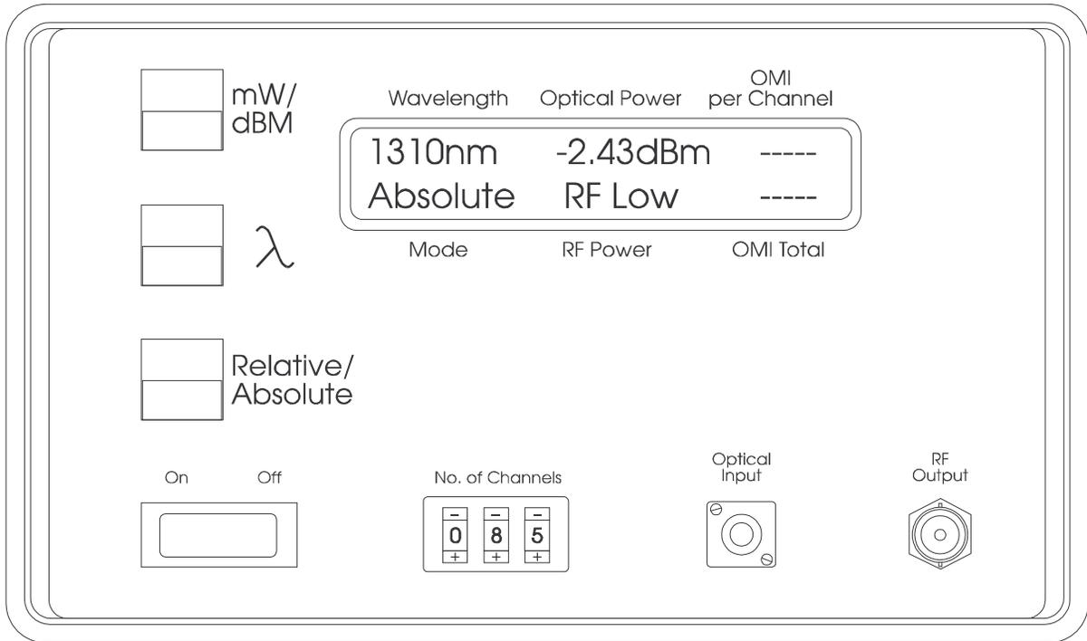
Figure 11 The FOS 1000A with RF Modulation Out of Range
