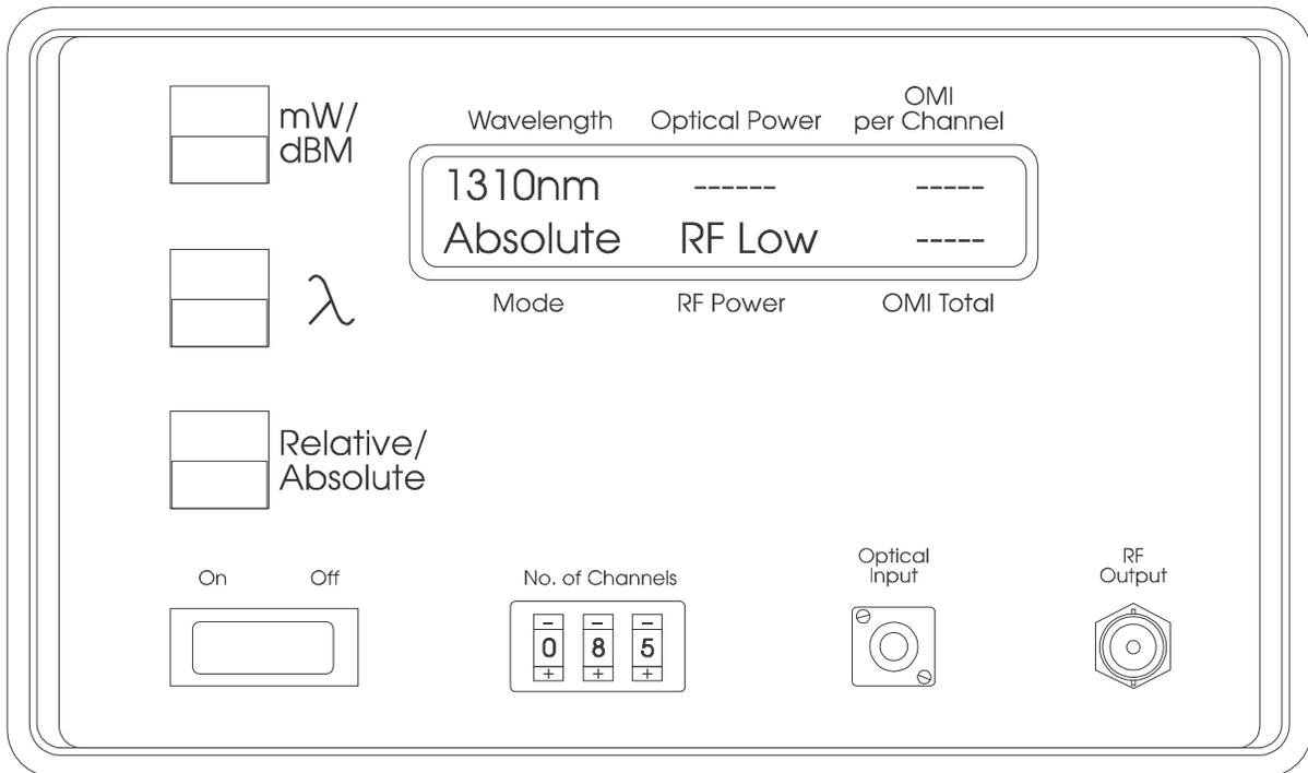
**Figure 4 The FOS 1000A Front Panel Controls and Indicators**
