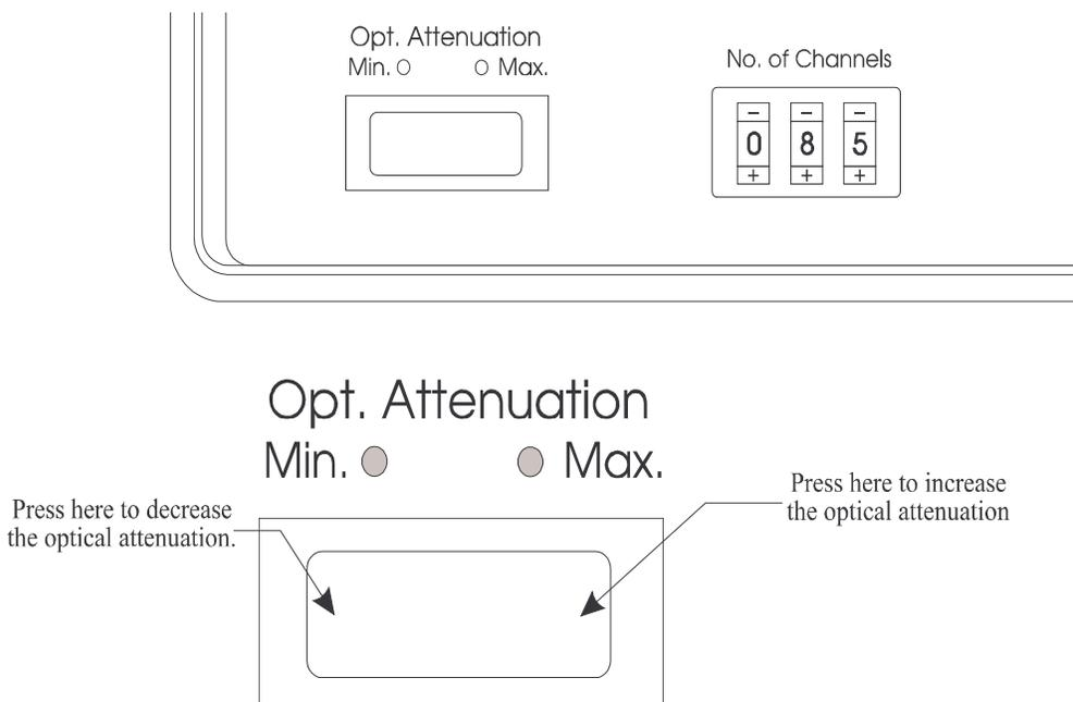
**Figure 13 The FOS 1000A Front Panel with optional Optical Attenuator**
