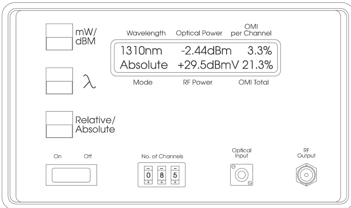
Figure 5 The FOS 1000A Default mW/dBM Selection
