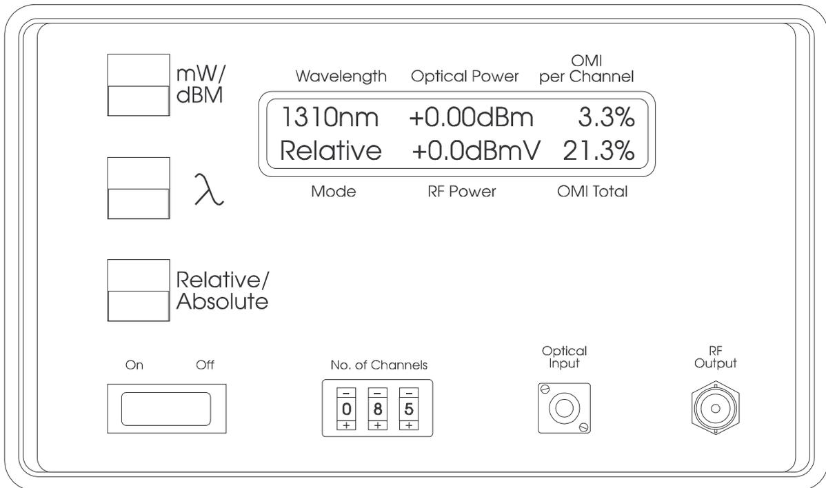
Figure 9 The FOS 1000A Relative Display Mode
