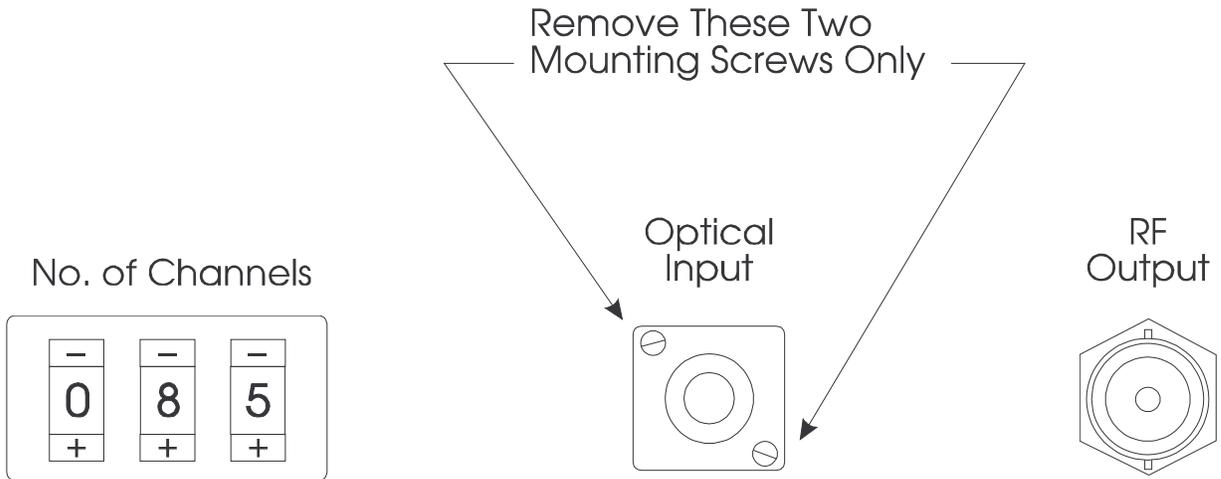
**Figure 12 Optical Interface Mounting Screws for Cleaning**
