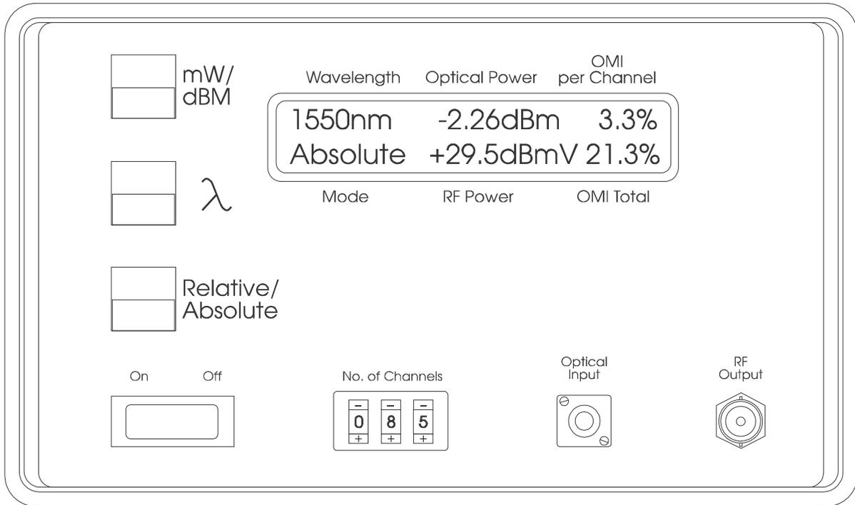
Figure 6 The FOS 1000A Wavelength Select Push-button
