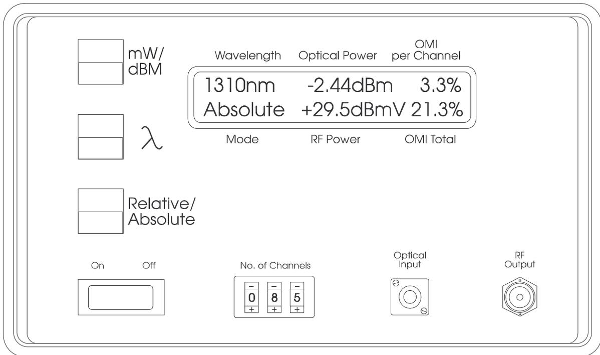
Figure 8 The FOS 1000A Normal Display Mode Absolute, 1310 nm
