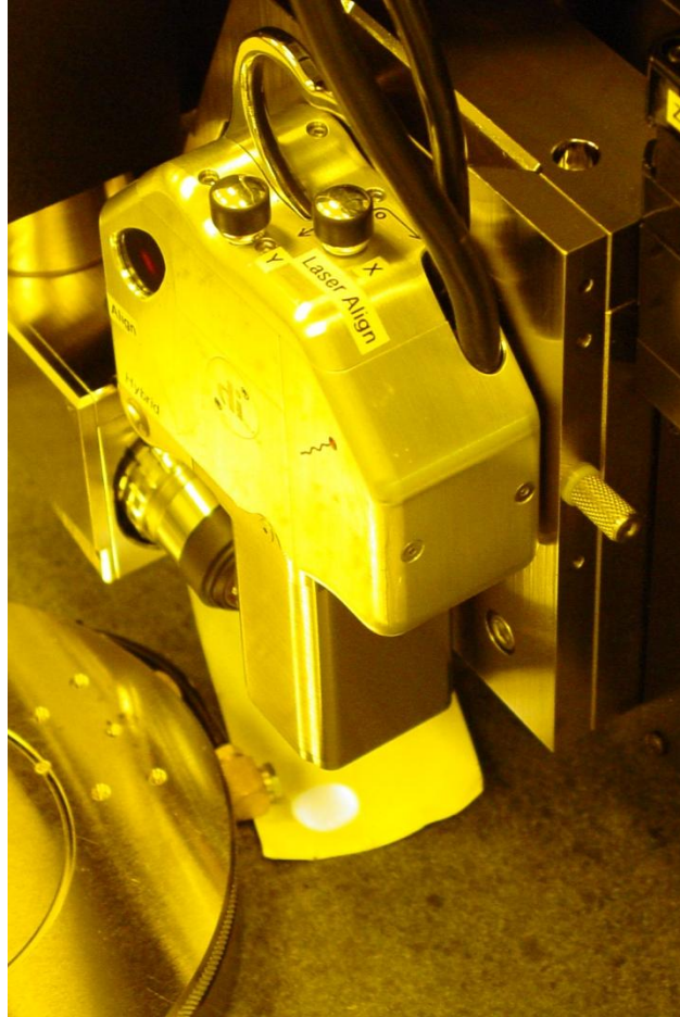
Figure 11. The stage position allowing the white light from the microscope to shine on the granite table to allow better alignment of the cantilever laser to the cantilever via shadow profile on the table. Note the white paper under the AFM head to improve visibility of the laser spot and cantilever shadow.
