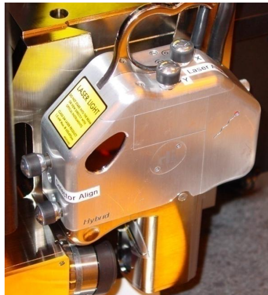
Figure 15. Side view from the Left of the AFM head showing the two knobs used to move the side mirror. Adjust them until the red dot on the screen lines up with the vertical gaps between the four sensors. A photograph of the AFM head is shown at the right.
