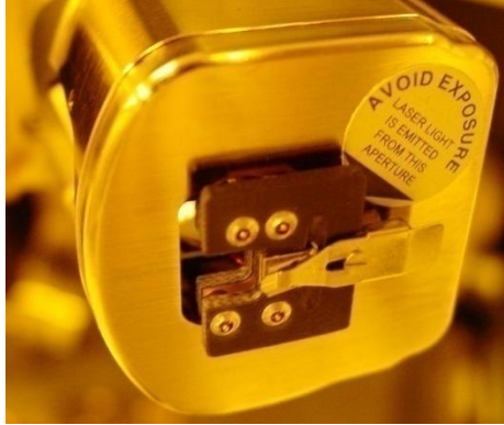
Figure 6. Disconnecting AFM head, placing the tip holder on pins, and remounting the AFM head. Note the asymmetric pin locations designed to allow the probe holder to fit only in the proper orientation. Make sure that the probe holder is seated flush against the head pin base, but be very gentle and do not push the pin base sideways – the z-piezo could break with excessive force. The video clip shows the mounting sequences. Note that the clamping screw for the AFM head has reverse threads – turn CCW to clamp the head and CW to release it.
