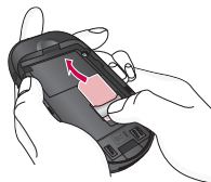
To remove the SIM card
