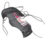
To insert the SIM card
