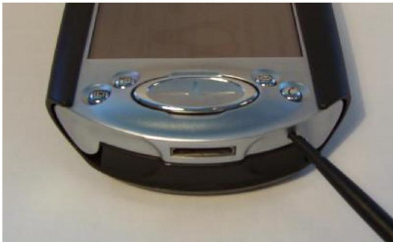
Figure 4-1: Resetting the MBU
