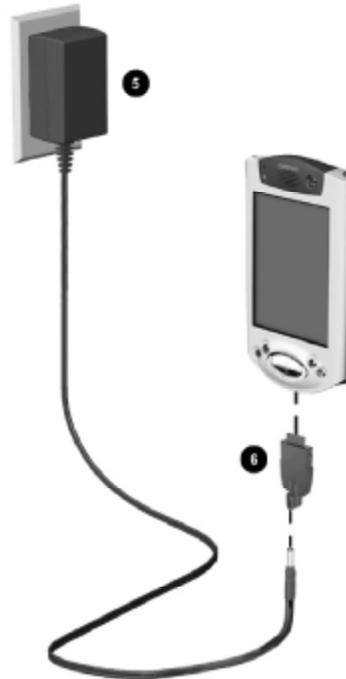
Figure 2.15: Insert the AC adapter into the DC adapter plug
