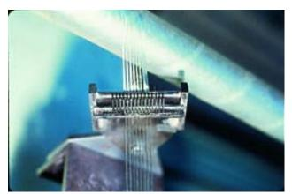
FRP materials are products of both the raw materials and the construction process used. The most commonly used processes for producing corrosion-grade FRP parts are filament winding, contact molding, centrifugal molding, matched die compression molding, and pultrusion.
