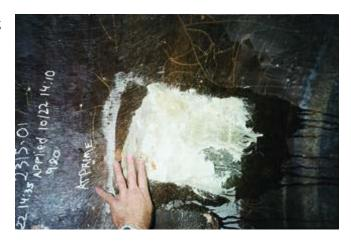
A 10" x 10" bond test patch is suggested, consisting of MMWRMWRM (M = 1.5 oz random chopped mat, WR = 24 oz woven roving). This assures that the patch is large enough for evaluation and stiff enough to peel at the bond plane if the bond is weak. Tape is left under one edge of the patch to start the peeling.
