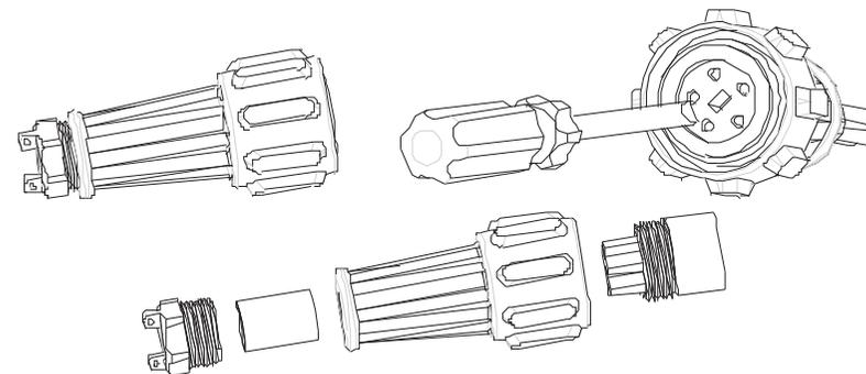
2) Connect 5 cables into their respective channels on the AC terminal, while 'N' represents Neutral, '1, 2, 3' represent 3 line channels and 'E' is ground, tighten all screws (1.0Nm (9 lbf.in.) max).
