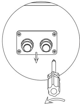
2. Slightly loosen the swivel nut, remove the filler-plug from the M16 cable gland.
