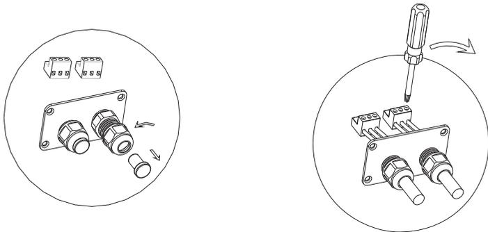
3. Make the cable through the hole of cable gland and put the cable into the RS485 terminals, fix all cables with screwdriver ('1' to '1', '3' to '3', '2' to the shielding layer)
