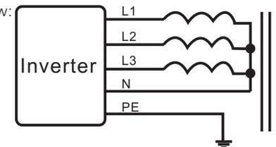
N of transformer should not be connected to PE.
