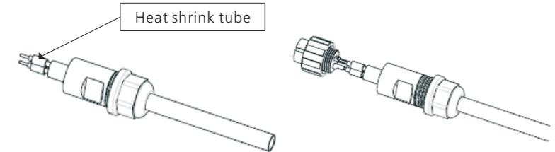
4. Insert the two metal head into relevant small cupreous hole, and fasten the connection by soldering.
