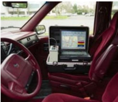
**Drive Test System in Vehicle**
