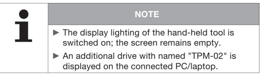
Copy the new firmware into the root directory of the "TPM-02" drive on the PC/laptop.
