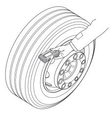
Move the hand-held tool along the side wall of the tire according to the speed of the animation.
