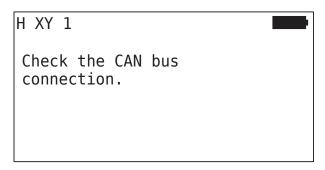
Check CAN bus communication to the components (CCU, display and CAN switch).
