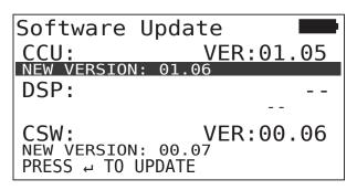
Press the Return key to start software transfer for the CCU.
