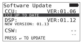
Press the Return key (a) to start software transfer for the display.
