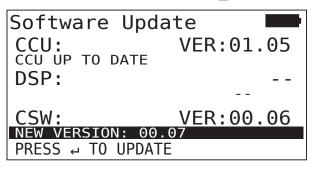
Press the Return key to start software transfer for the CSW (switching module).
