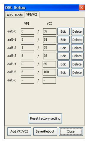
Enter the interface, the instrument will display former 8 series of VPI/VCI parameters, you can revise any series of VPI/VCI according to your requirement, input VPI/VCI revised value in the VPI/VCI input bar, and press reset setting key, the new value will generate(not lost even if power off)
