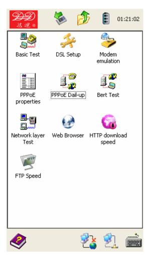
xDSL test function includes: physical layer test, DSL parameter settings, Modem emulation, PPPoE properties, PPPoE dial-up, ATM loopback test, network layer test, Web Browse,
