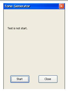
The device can send the audio signal at the end of twisted-pair, use Tone Tracer to find the compatible line pair at the other end.
