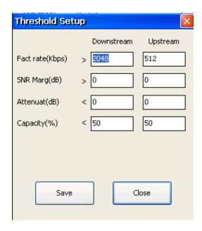
Click Result to enter Result estimate window, you can set up line parameters and threshold value to decide if the line is qualified, as follows:
