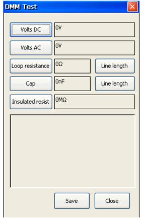
Then connect test line, click the test items to start the testing. All test items introduced as below.
