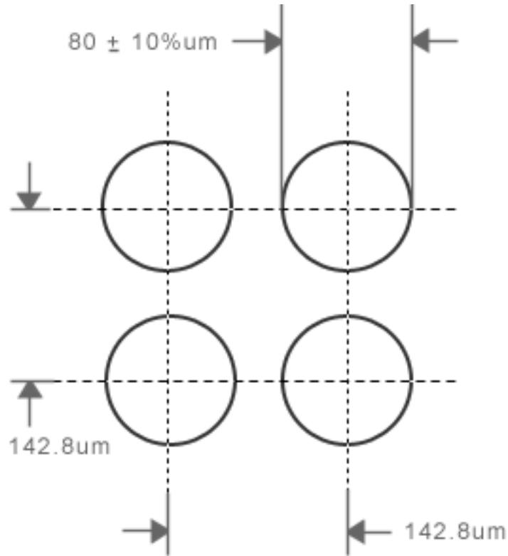
**Figure 3: OneArray<sup>®</sup> Glass Slide with Spotted Probe Region.**
