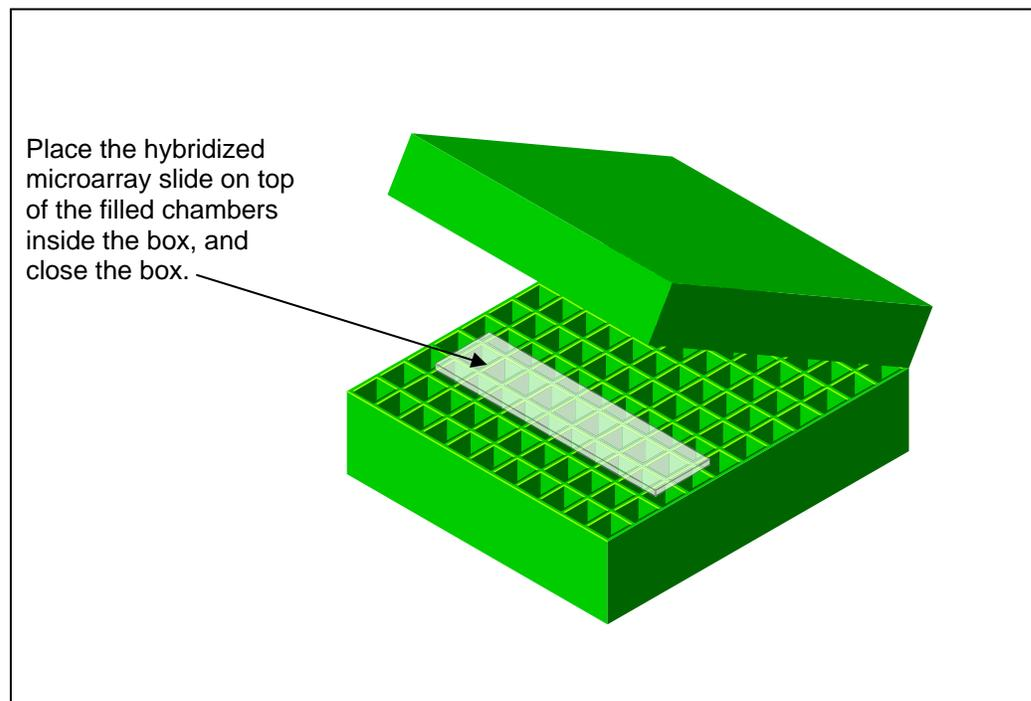
**Figure 2: Step 4A(iii) → aRNA Hybridization—Glass Slide Inside Chamber Box<sup>2</sup>**
