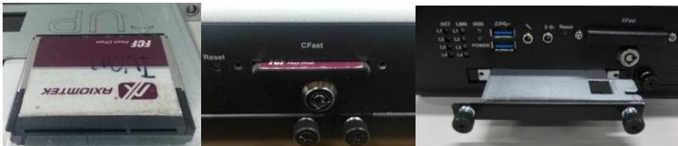
**Step 4** Fasten screws of HDD/CFast bracket
