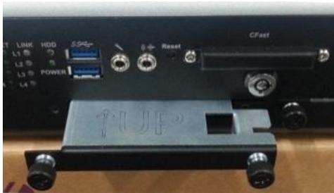
**Step 2** Assemble the HDD/SSD bracket together with the SATA HDD/SSD
