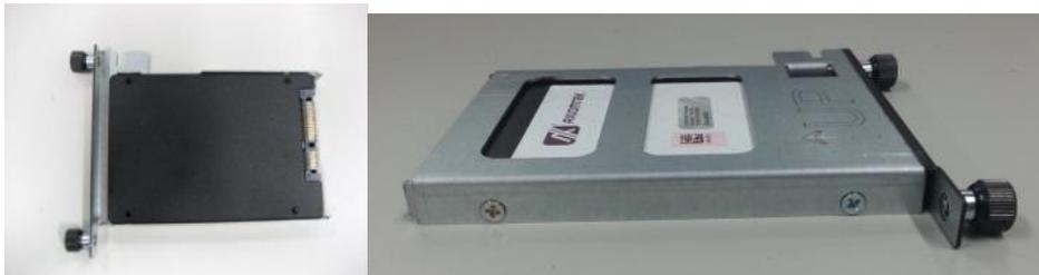
**Step 3** Slide CFast card or HDD/SSD into slot cautiously
